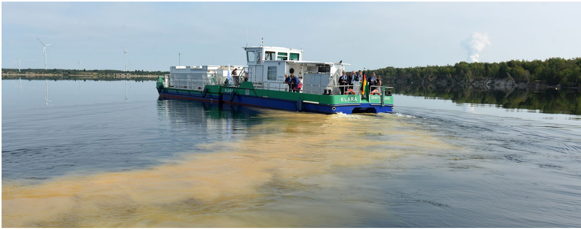
Fig. 3 Water treatment at Lake Partwitz showing brown colored water due to iron buffering (image provided by LMBV)
