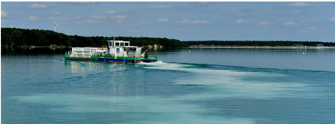
Fig. 4 Water treatment at Lake Partwitz showing a turquoise color due to aluminum buffering (image provided by LMBV)
