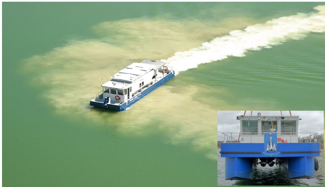
Fig. 11 Water treatment vessel “Barbara” in operation—showing the input system between the vessel’s hulls (image provided by LUG/LMBV)
