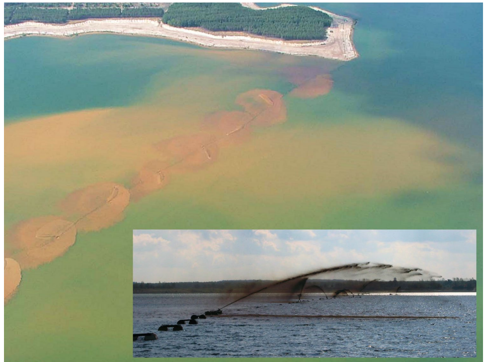
Fig. 5 Lake Geierswalde with sprinklers to distribute the suspended lime sediments (image provided by ETA/LMBV)
